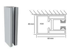
The guide rail is manufactured from extruded aluminium with a box section for fixing and high density 5mm pile brush seals. The H34 guide profile is supplied as standard. The rail must be rebated behind the outer brickwork to achieve maximum security.
