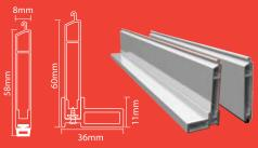
Extruded aluminium with reinforcing angle. Can be supplied with rubber base or reinforcing angle.
