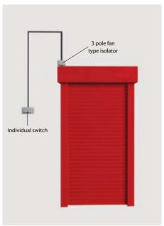
Control mechanisms are available as both single motor and group command activated motors for multiple shutters, so that shutters can be operated individually or in groups. Single rooms can be controlled individually, ensuring that the shutters are only operated in full sight of the user.
